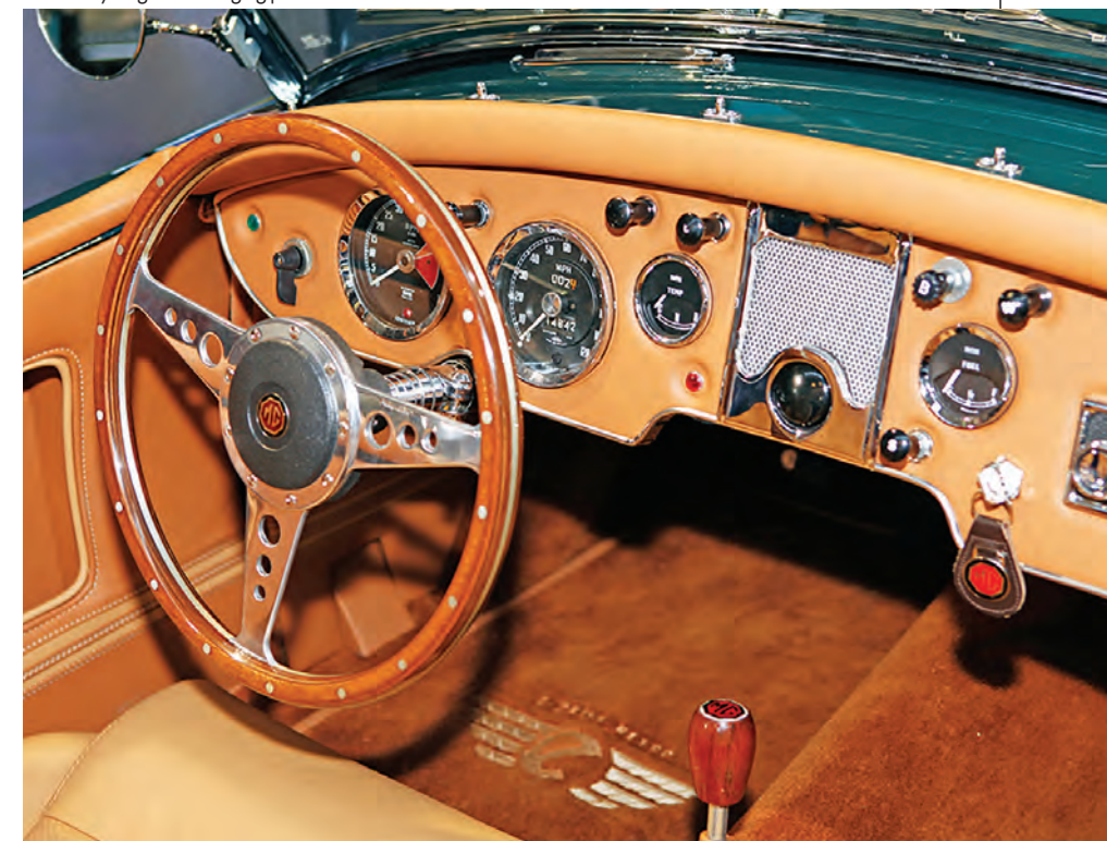
The dashboard still keeps its original configuration. The fuel gauge shows the status of the battery
